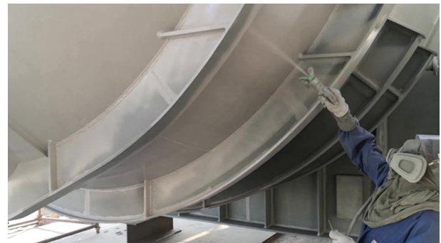
Fig. 4. Image of spray gun painting with a manually inserted green mark at the gun tip.
