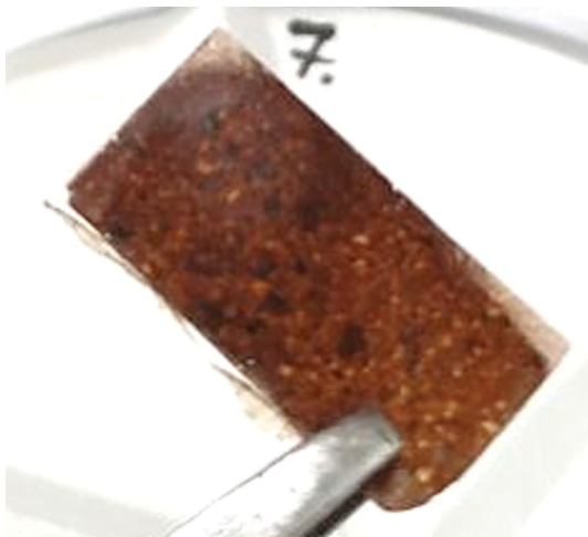
Fig. S3. Films prepared by hot pressing of PHB and OL (10% OL at 175^\circ\text{C} for 15 min pressed at 5,000 psig).
