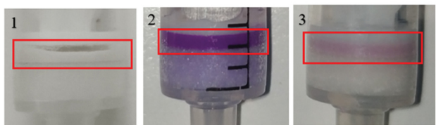
Fig. 8. ACPases immobilized on TOYO treated with Schiff's reagent. (a) ACPase from wheat germ; (b) ACPase from potato. 1: immobilized ACPases derivatives; 2: ACPases derivatives oxidized; 3: ACPases derivatives oxidized and reduced.
