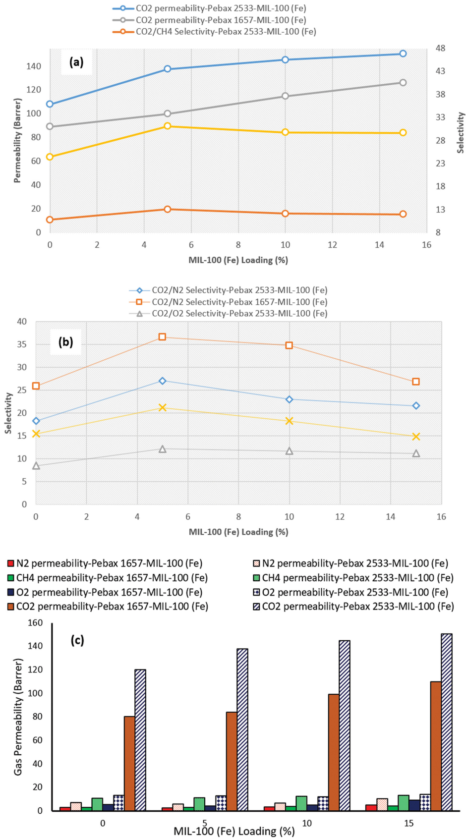
Fig. 5. Comparison of the separation performance of PEBAX1657/MIL-100 (Fe) and PEBAX2533/MIL-100 (Fe) membranes due to increasing loading percentages of MIL-100 (Fe); (a) CO 2 permeability and CO 2 /CH 4 selectivity at pressure of 5.5 bar (b) selectivity of CO 2 /N 2 and CO 2 /O 2 at pressure of 5.5 bar. (c) Permeability of CO 2 , CH 4 , N 2 and O 2 at a pressure of 3.5 bar.
