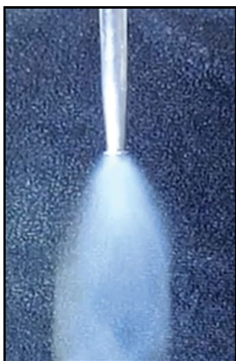
Fig. 3. Spray generated using the ultrasonic atomizer.
