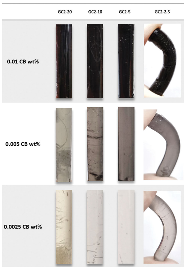
Fig. 5. CB/DCPD sticks obtained after FP with different contents of CB and catalyst.
