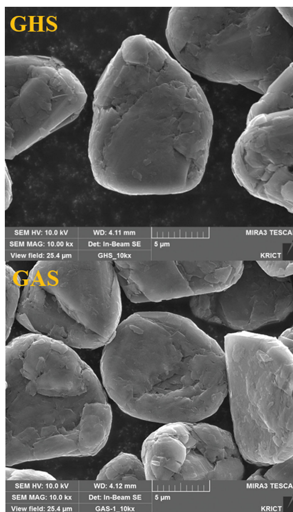
Fig. S2. SEM images of GHS and GAS.
