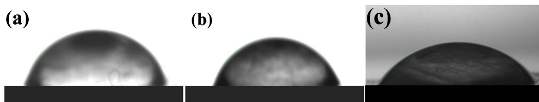
Fig. 5. Water contact angle photographs of (a) PVDF membrane, (b) GO/PVDF membrane, (c) LiI-NcMs.
