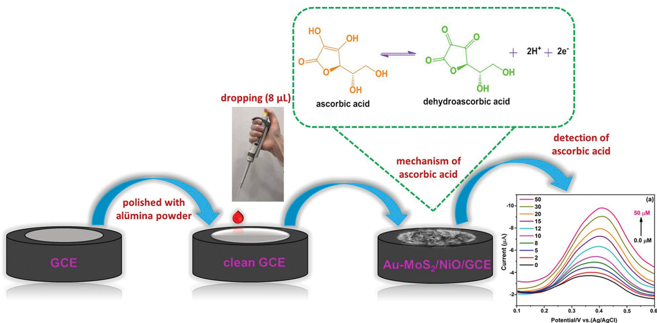
Scheme 2. The fabrication of Au-MoS 2 /NiO composite on GCE for AA detection.
