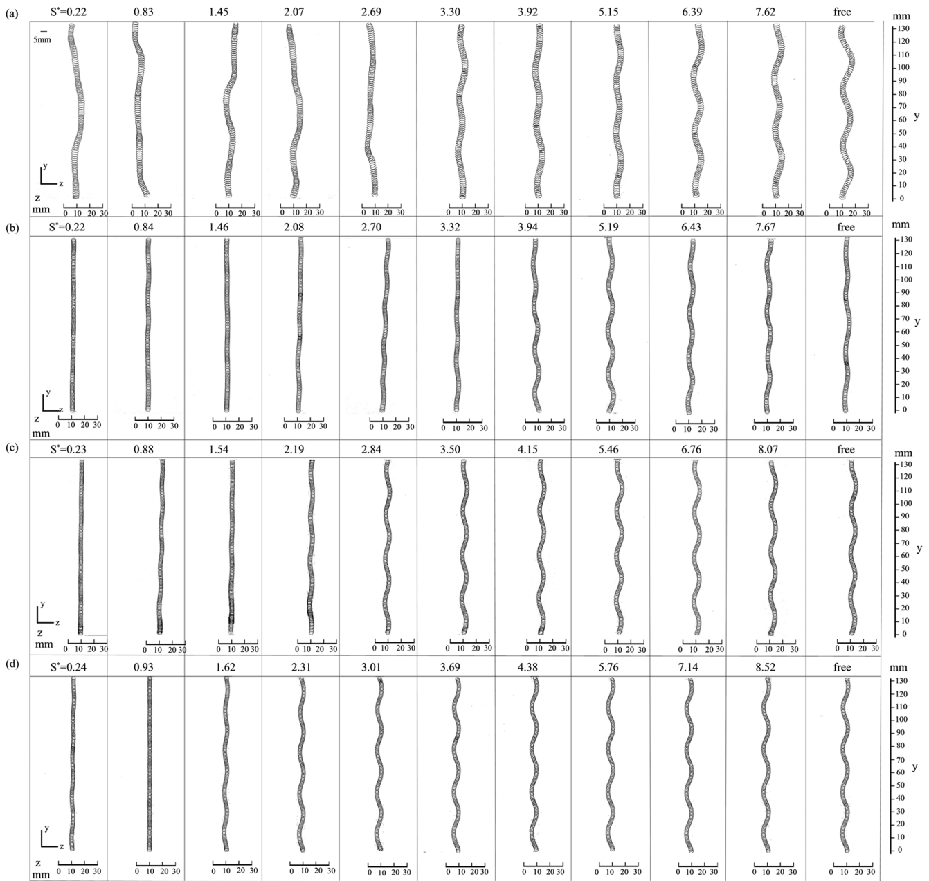
Fig. 4. Effect of different surfactant concentrations on the trajectories of rising bubbles in the y - z plane: (a) pure water, (b) 100 ppm, (c) 400 ppm, and (d) 800 ppm.
