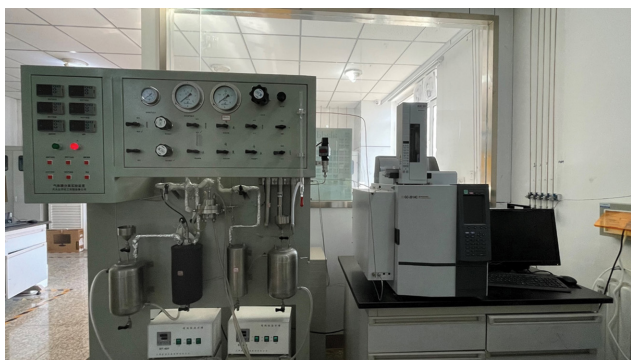
Fig. S1. The real picture of the self-built permeation measurement equipment for gas permeation.
