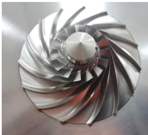
Fig. 1. IET supercritical CO 2 centrifugal impeller (Zhu et al. [29]).
