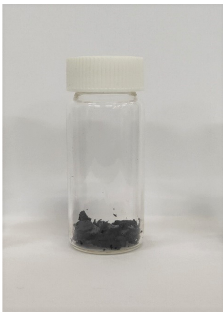
Fig. S1. Solid humins collected from the bottom of the reactor after 2 hours of reaction obtained under condition of 180 °C, 0.15 ml sulfuric acid, 2 ml of ethanol, 80% moisture content.
