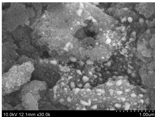
Fig. S2. SEM image of Cu-Ni(1:1)/AC catalyst.
