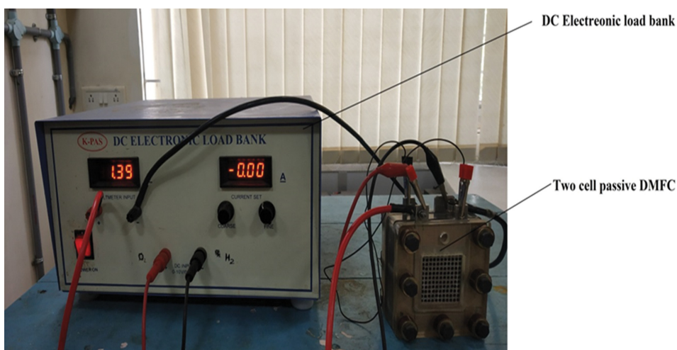
Fig. 1. Assembly of two cell passive DMFC stack. (1) and (7) Cathode end plates (2) and (6) Cathode current collectors, (3) and (5) Anode current collectors, (4) Methanol reservoir.
