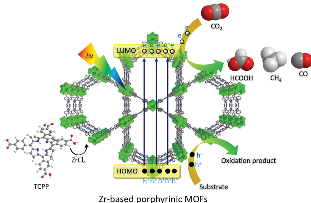
Fig. 17. Process of photocatalytic CO 2 reduction over Zr-based porphyrinic MOFs.
