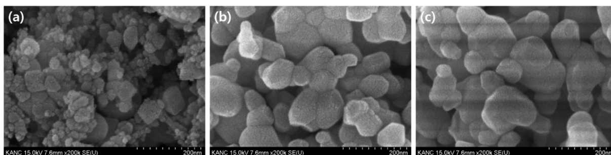
Fig. 3. SEM image of (a) pure \text{SnO}_2 , (b) 6 wt% CuO and (c) 35 wt% CuO combined \text{SnO}_2 .
