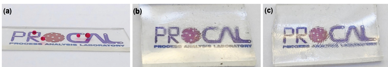
Fig. S2. Pictures of PDMS that are exposed to the heat with the distance of (a) 5 mm, (b) 3 mm and (c) 7 mm. Red water droplets were placed on 5 mm sample to show that the sample is surface-treated. Cracks and wrinkles from sudden temperature change caused 3 mm and 7 mm samples to become translucent.
