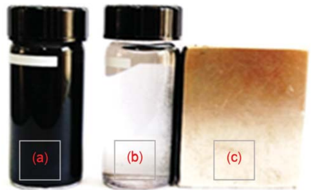
Fig. 5. The separation of the AC-Fe 3 O 4 from the solution: (a) is solution before separation of AC-Fe 3 O 4 , (b) solution after separation of AC-Fe 3 O 4 and (c) external magnetic.
