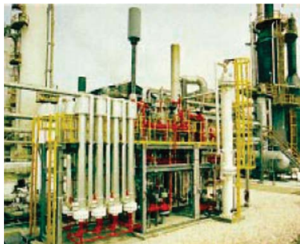
Fig. 1. Photograph of two stages H 2 separation system (obtained from PRISM ® brochure) in ammonia installation. Reprinted with permission from ref [28], Copyright 2009 American Chemical Society.
