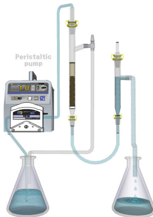
Fig. 2. Schematic diagram of column-type packed-bed adsorption reactor.
