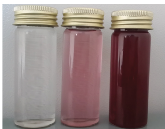
Fig. 13. The photographs of (right) feed solution, (middle) permeate of M_0 membrane and (left) permeate of M_1 membrane.
