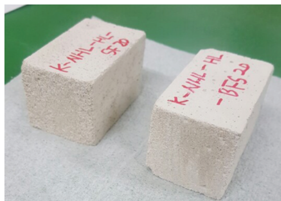
Fig. 7. Photograph of hardened K-NHL_HL_BFS20 and K-NHL_HL_SF20 mortars after 28 days.
