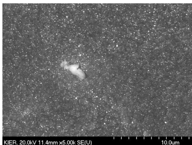
Fig. 3. The surface SEM analysis of Pd-Ru membrane after MSR: white spots are dust of alumina catalyst.
