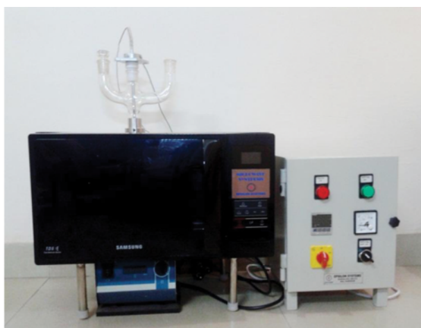
Fig. 1. Experimental setup of microwave reactor.
