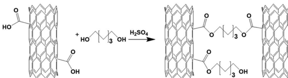
Fig. 1. Esterification reactions between carboxylic acids on the CNT and the alcohol groups of the linker (1,5-pentanediol), resulting in chemical links between individual CNTs. Both cross-linking and one-side reactions are present in the product.
