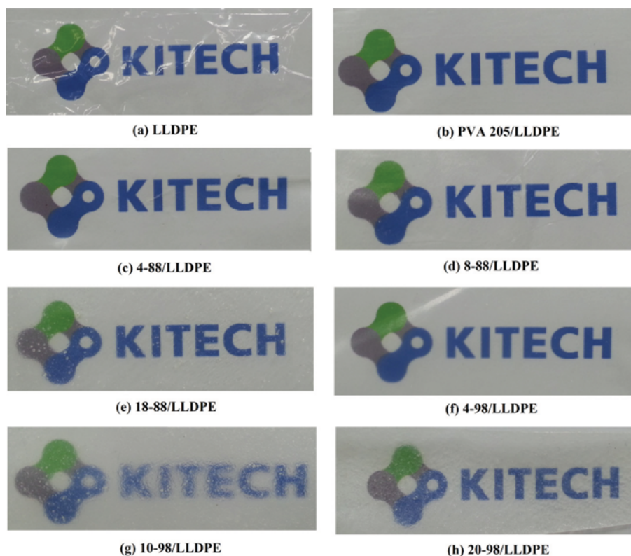
Fig. 3. Photograph images of the PVA/LLDPE composite films on colorful text.
