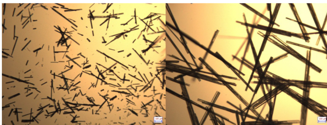
Fig. 11. Results of linear cooling strategy (20 °C/hr) (Left: with industrial seed preparation, right: with optimal seed preparation).
