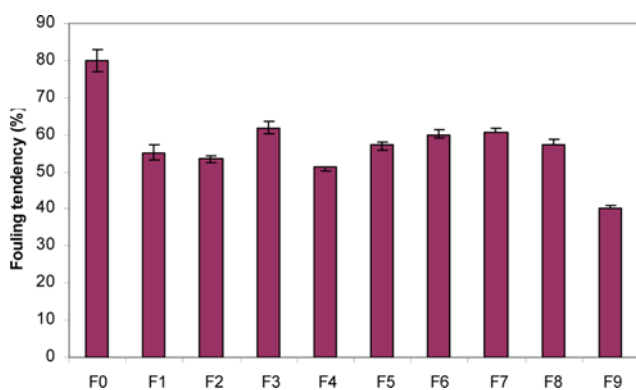
Fig. 9. Fouling tendency of the prepared thin layers.
