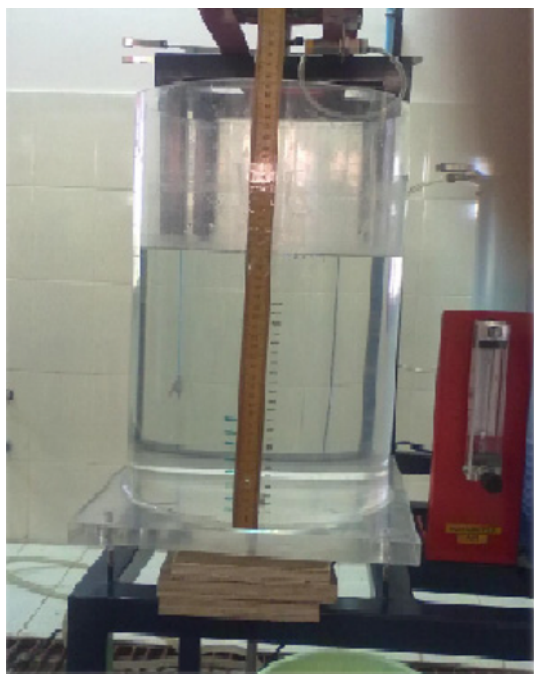
Fig. 1. Gravity-Driven Method (Reynolds number range-15000-35000 for water as a function of pipe diameter).
