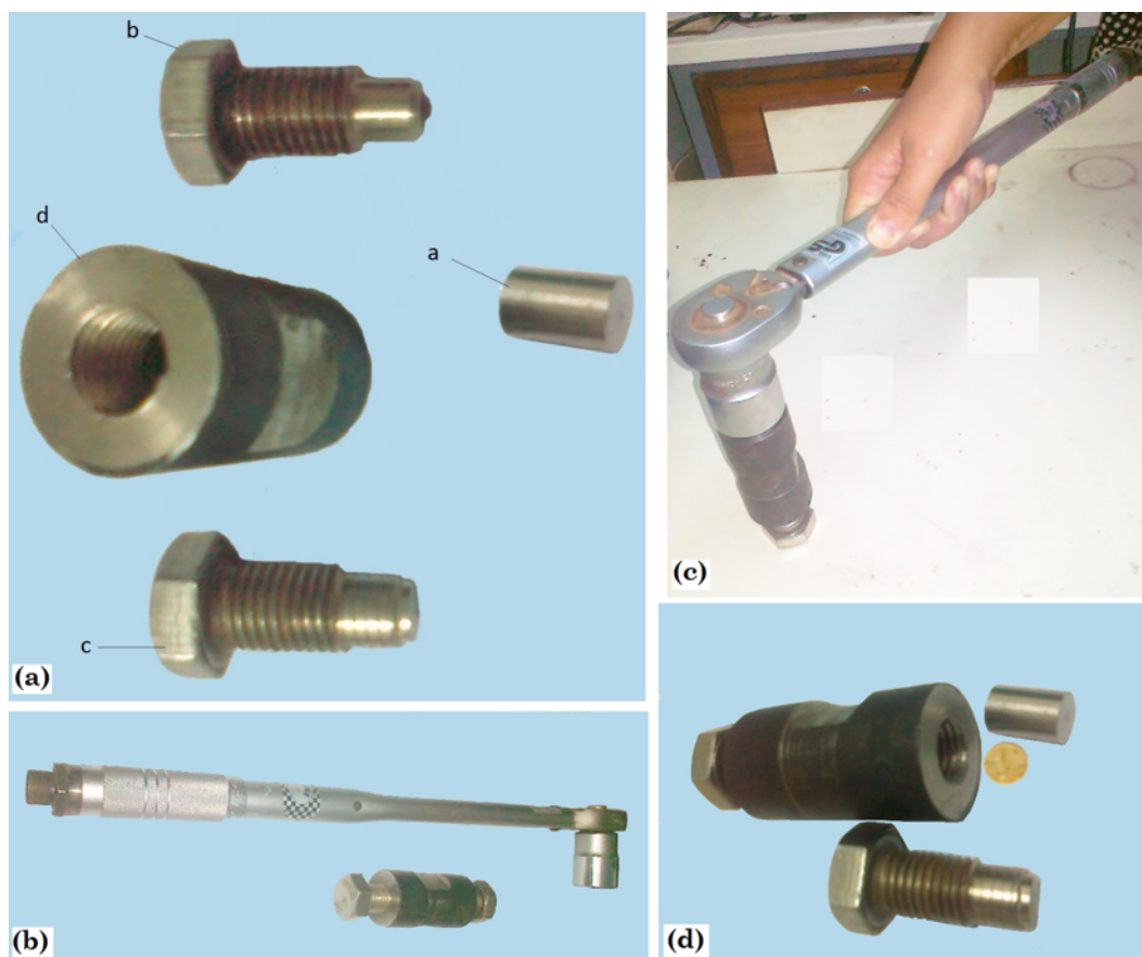
Fig. 1. Pellet formation (a) Self-designed mechanical tool for pellet formation; (b) Torque wrench and self-designed mechanical tool for pellet formation; (c) Pressure being applied with a torque wrench; (d) Pellet formed using the self-designed assembly.
