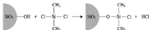
Fig. 2. Silanization reaction of fumed silica with DMDCS.
