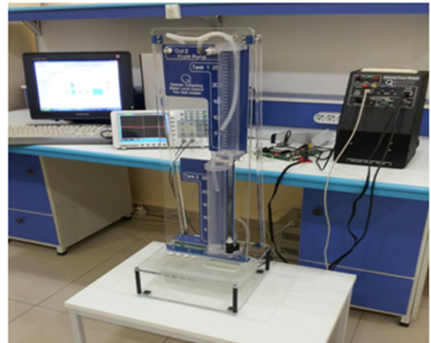
Fig. 4. The coupled tank experimental setup.
