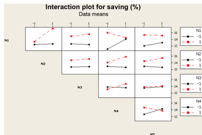
Fig. 9. Effect of main design variables', N1, N2, N3, N4, and N5, interactions on TAC saving.
