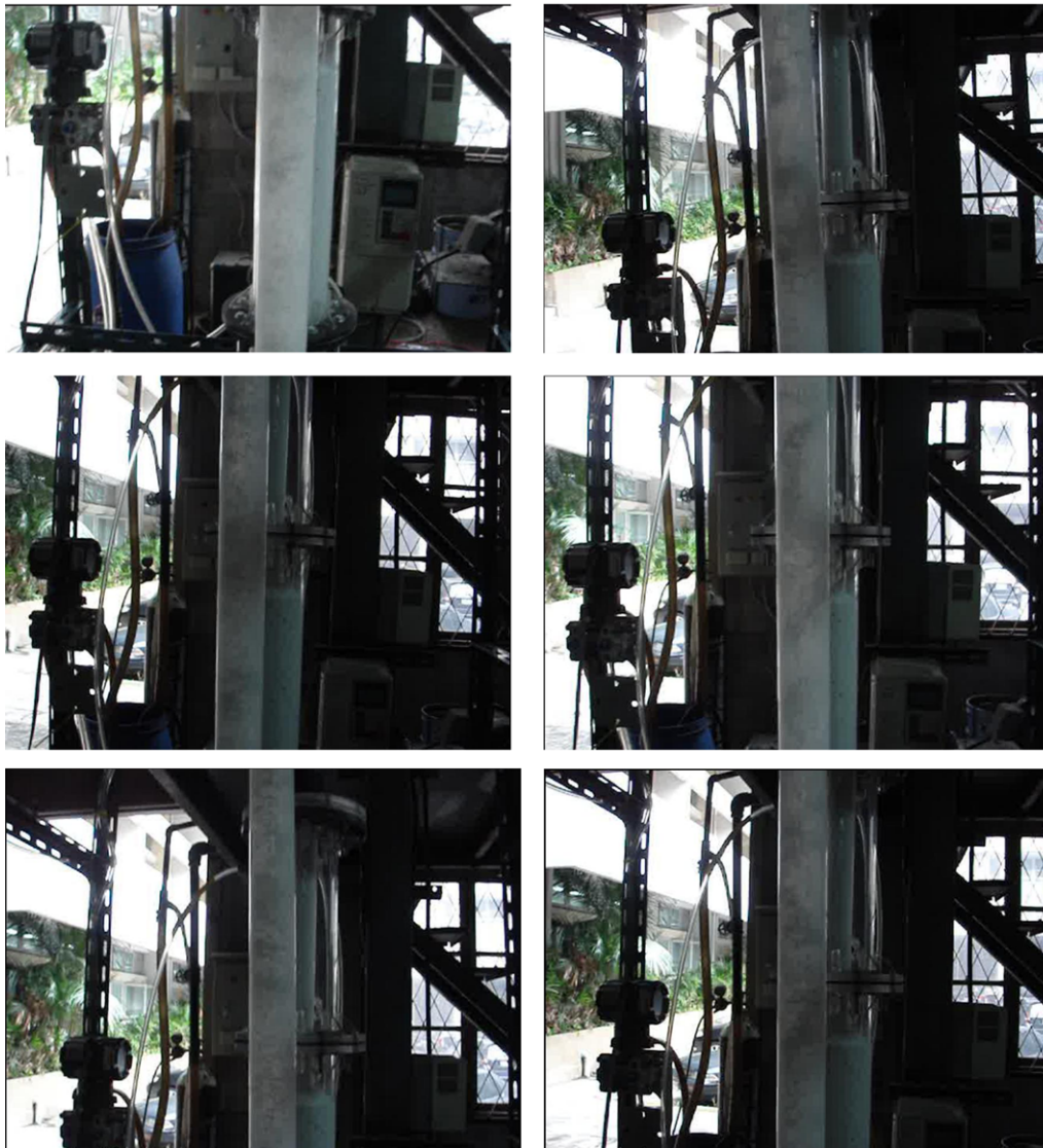
Fig. 9. c. The snapshots from the CFB experiment in the laboratory demonstrating the slug flow pattern inside the column.
