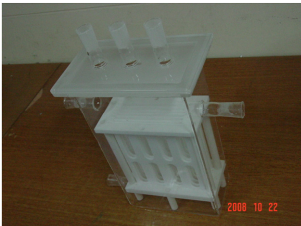
Fig. 2. Circulating flow reactor with Teflon supporter.
