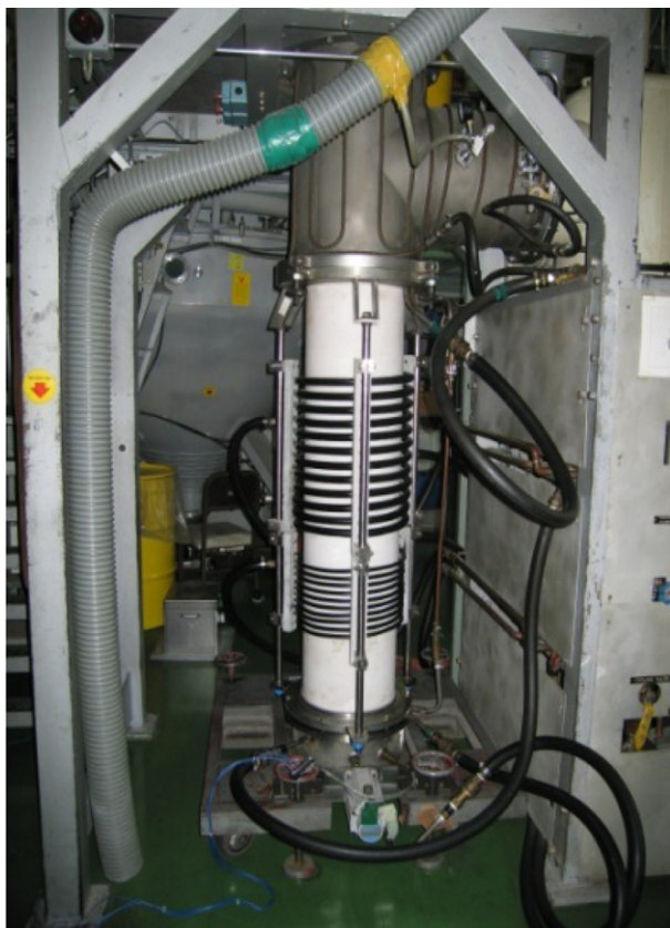
Fig. 1. Experimental apparatus (with high frequency induction coil generator).
