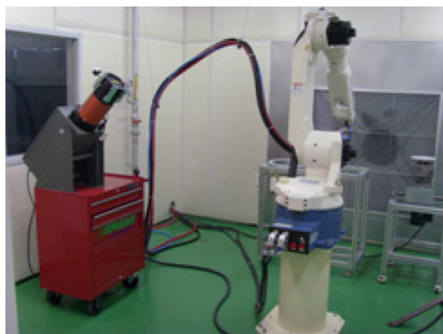
Fig. 2. Plasma spraying equipment for plasma spraying coating.
