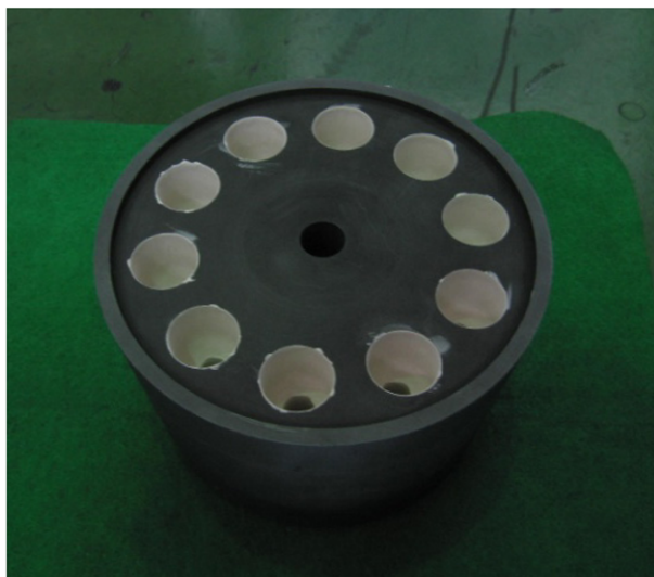
Fig. 4. Molds of graphite crucible for the reaction between ceramic coating materials and uranium.
