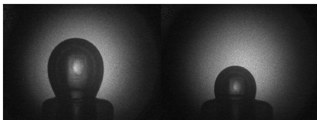
Fig. 2. Bubble images captured at 0 second and 1,080 seconds at 310 K.
