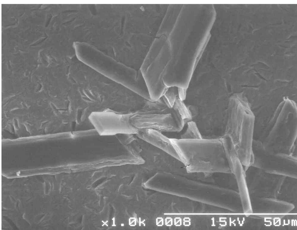
Fig. 9. A SEM photograph of triclinic crystalline formed from a slow cooling crystallization of cupric sulfate (Run-3).
