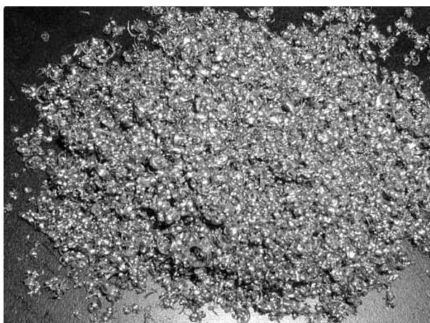
Fig. 1. Iron scrap used in this study. This material was obtained from a metal-processing facility and acid washed before use to remove cutting oil on the surface.
