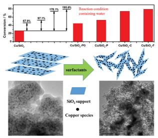
The addition of surfactants could increase copper dispersion, decrease particle size and produce many pores to provide more chances for reactants to touch active sites so that the negative effects of water can be counteracted.
