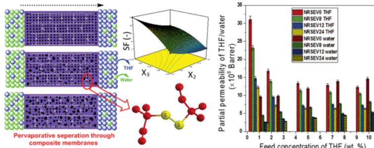
Accelerated sulfur vulcanized and filler incorporated composite membrane intrinsic properties are found to vary with concentration, temperature and filler towards recovery of hazardous THF. Excellent balance of flux and separation factor is also observed by response surface methodology design.
