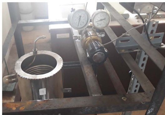
Fig. 3. The modified pressure regulator to control the pressure in the reactor and the pressure out of the reactor.
