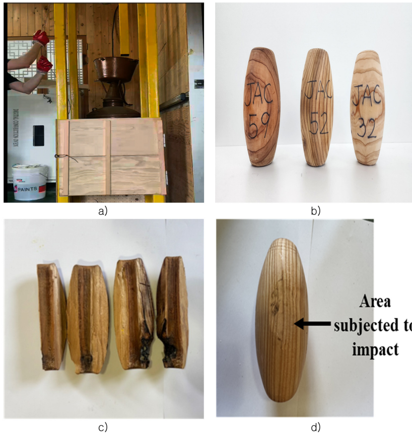
Fig. 13. Images of a) testing equipment and b) wooden marine buoys used for determining impact resistance, c) testing results of wooden marine buoy processed in the c) longitudinal and d) horizontal directions.
