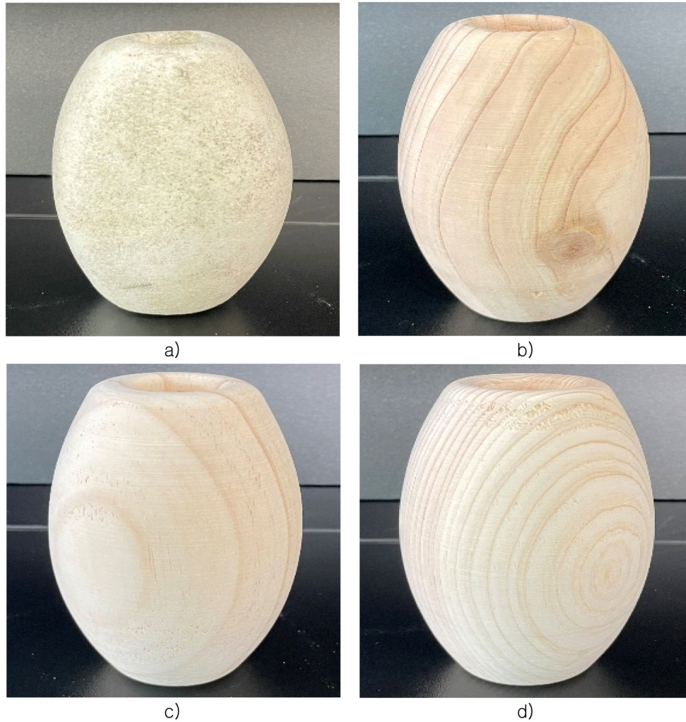
Fig. 1. Images of marine buoy made with a) polypropylene, b) Japanese cedar, c) radiata pine and d) Japanese cypress.
