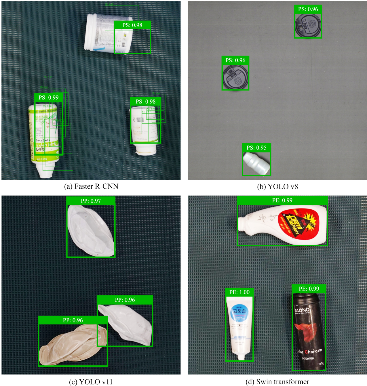
Fig. 5. Bounding box and confidence score visualization of waste plastic detection by models [28].
