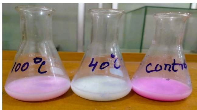
Fig. 4. Confirmation of purified lipase with full cream milk after purification with chromatography.
