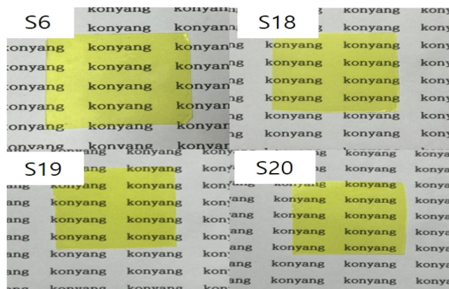
Fig. 9. Photographs of coating films prepared with different amounts of benzophenone.
