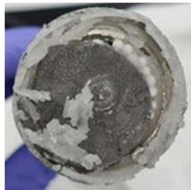
Fig. 3. Images of blocked reactor after the heating of as-received reactant.
