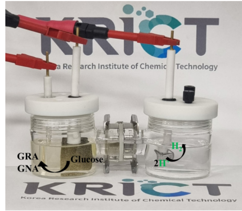
Fig. 3. The glucose electrolysis experiments were conducted in an H-type electrochemical cell, in which the anode electrolyte was 1 M of KOH solution dissolved with glucose (100 mM), and the cathode electrolyte was 1 M KOH, and an anion-exchange membrane.
