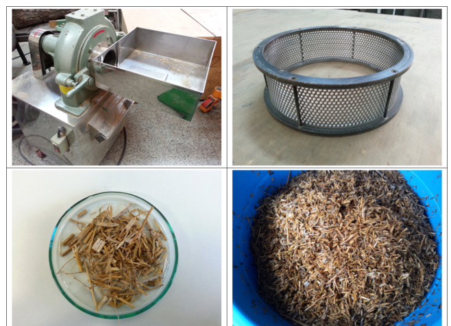
Fig. 1. Images of milling machine (top-left), screen used in the machine (top-right), grounded rape stalk (bottom-left), and the rape stalk completed immersion treatment (bottom-right).
