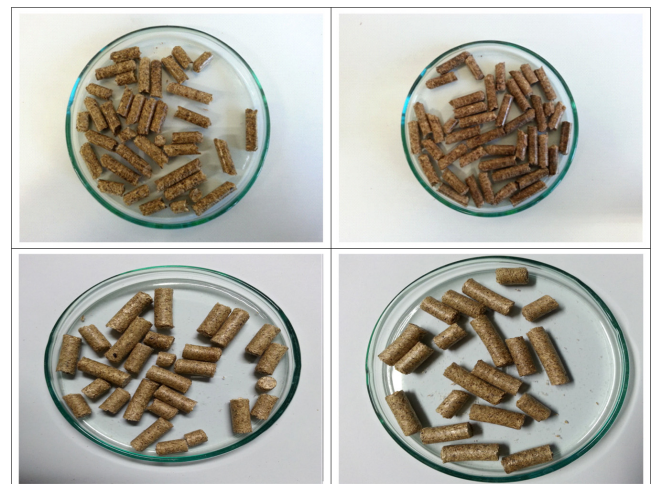
Fig. 3. Images of non-woody pellets produced with 100 wt% non-immersed rape stalk (top-left), 90 wt% larch sawdust/10 wt% non-immersed rape stalk (top-right), 10 wt% larch sawdust/90 wt% immersed rape stalk (bottom-left) and 20 wt% larch sawdust/80 wt% immersed rape stalk (bottom-right).
